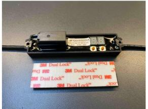
The 8amp relay is very vibration sensitive. Insulate the module from engine and chassie vibrations!!!!
