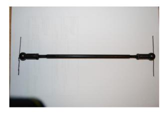
Remove stock shiftrod and measure.
